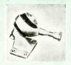
A modern engine support unit employing rubber vibration isolating construction. Applied to all types of aircraft installations by modifications of components. They feature: low weight, simplicity of installation and inspection, built-in damper and interlocking parts. Standard
