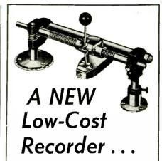
This is a new type of instantaneous recording mechanism, by which exceptional quality recordings may be made by inexperienced operators. Adaptable to any height recording turntable. Simple lever arrangement allows engaging of feed screw and lowering of cutting head at the same time. Cutting pitch is 110 lines per inch, outside-in, with provision for making "run-out" grooves. Thumbscrew allows adjustment of cutting depth.
