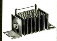
Bradley selenium rectifiers give good efficiency and stability for medium voltage power applications at D.C. ratings up to 24 volts and at current ratings up to 5 amperes per plate. Ratings are for continuous operation in naturally circulating air at 35°C. ambient.
