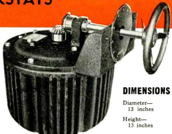
As noted, increased capacities of air-cooled POWER-STATS are possible by oil-immersion. For a high continuous output from a unit of small physical size, SECO offers its standard 1126 and 1226 types in a compact, cast-aluminum oil-container. They may also be used in hazardous or humid atmospheres and where high momentary overloads are occasioned.
