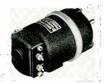
"FB" FRAME, 21/4" x 4". DC—as wound field and permanent-magnet field motors and generators, and servo motors. AC—as universal motors, and permanent-magnet generators, one, two, or three phase. Also in shorter length; as capacitor start and run, two and four pole AC motors. As induction type to 1/200 HP at 3400 RPM; as synchronous type to 1/500 HP at 3600 RPM.
