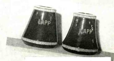
All Lapp footing and guy insulators incorporate the Lapp patented curved-side compression cone {right}. With the same dimension and same wall thickness, the curved-side cone has double the strength of the straight-side cone {left}.
