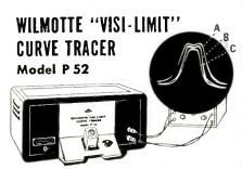
For rapid alignment of 1.F. coils of frequencies from 85 kc to 11 mc. Operator adjusts test trace (B) to fall between traces of limit coils (A and C), set up to production specifications. Defective coils immediately detected. All error is eliminated as circuit changes or line voltage variations affect all three traces equally.
