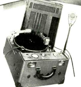
PRESTO MODEL K dual speed recorder, playack PA system, 12 inch turntable.
