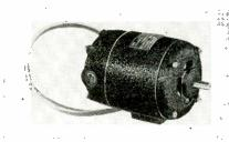
ALC FRAME, 3.9% x 51/16", internal fan cooled. As DC shunt, series, or split-field motors, to 1/15 HP at 3400 RPM. As servo motors; as universal motors to 1/10 HP at 6000 RPM.
