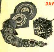
Featuring extremely low and uniform contact resistance and low noise level. Daven switches are supplied in varied combinations of decks, poles per deck and contacts per deck. Heavy duty, laminated, self-wiping arms need no lubrication; switch contacts and arms are of a special silver alloy lother metals to your specifications); bakelite or ceramic panels; breakbefore-make or make-before-break wiring.
