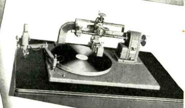
PRESTO 14 A studio recorder, directly gear driven at 78.26 and 33.3 r.p.m., selection 10 cutting pitches 88.136 lines per inch, designed to cut vertical or lateral masters or instantaneous recordings,
