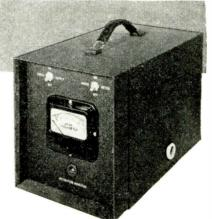
within a small percentage of error. Oscilloscope connection permits checking initial installation, trouble shooting the engine, detecting and eliminating costly errors due to worn or malfunctioning engine parts. Can be used in flight or on test stand: KM-1 for single cylinder aviation fuel engines, KM-2 for multicylinder engines, KM-3 automotive Fuel Test, KM-4 Automotive Road Test. Refer to Publication 23-82.
