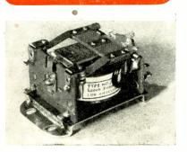
Typical of a wide variety of control relays, manufactured as standard, or to fit customer specifications, the illustrated No. 1127 metal base relay is an exceptionally fast-acting type, and can be used for keying low power radio transmitters. Made for either AC or DC, with contact arrangements up to 4 PDT; they are durable, and can withstand long cycling operations. Coil consumpition is 1.5 watts DC or 6 V/A 50-60 cycles, AC.
