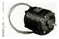
ALP FRAME, 3-%" x 4-5/16", capacitor start and run, two and four pole AC motors, internal fan cooled. As induction type to 1/20 HP at 3400 RPM; as synchronous type to 1/40 HP at 3600 RPM.
