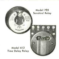
Model 705 Sensitrol Relay combines high sensitivity and high contact capacity. Positive operation on values as low as 2 microamperes or 1 millivolt d-c, or 10 microamperes a-c. Magnetic contact principle assures perfect contact and eliminates chattering. Also time delay and power relays designed to operate from WESTON sensitive relay contacts, providing complete control sequence.
