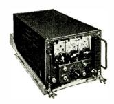
**AVIATION RADIO:** The Western Electric ARC-1 is a VHF transmitter-receiver for communications between planes and ground stations.
