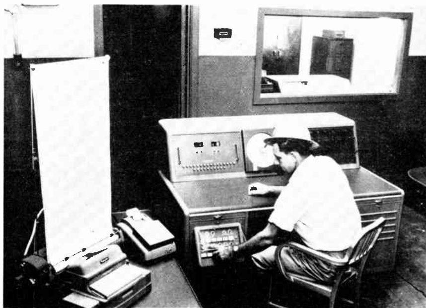
General-purpose digital computer is measuring 160 variables in Esso catalytic cracking unit. Twenty-seven of the variables are computed operating guides, such as catalyst circulation rate, carbon burning rate, material balance. Leeds & Northrup system now aids operators in process performance but in future, loop may be closed for completely automatic processing
