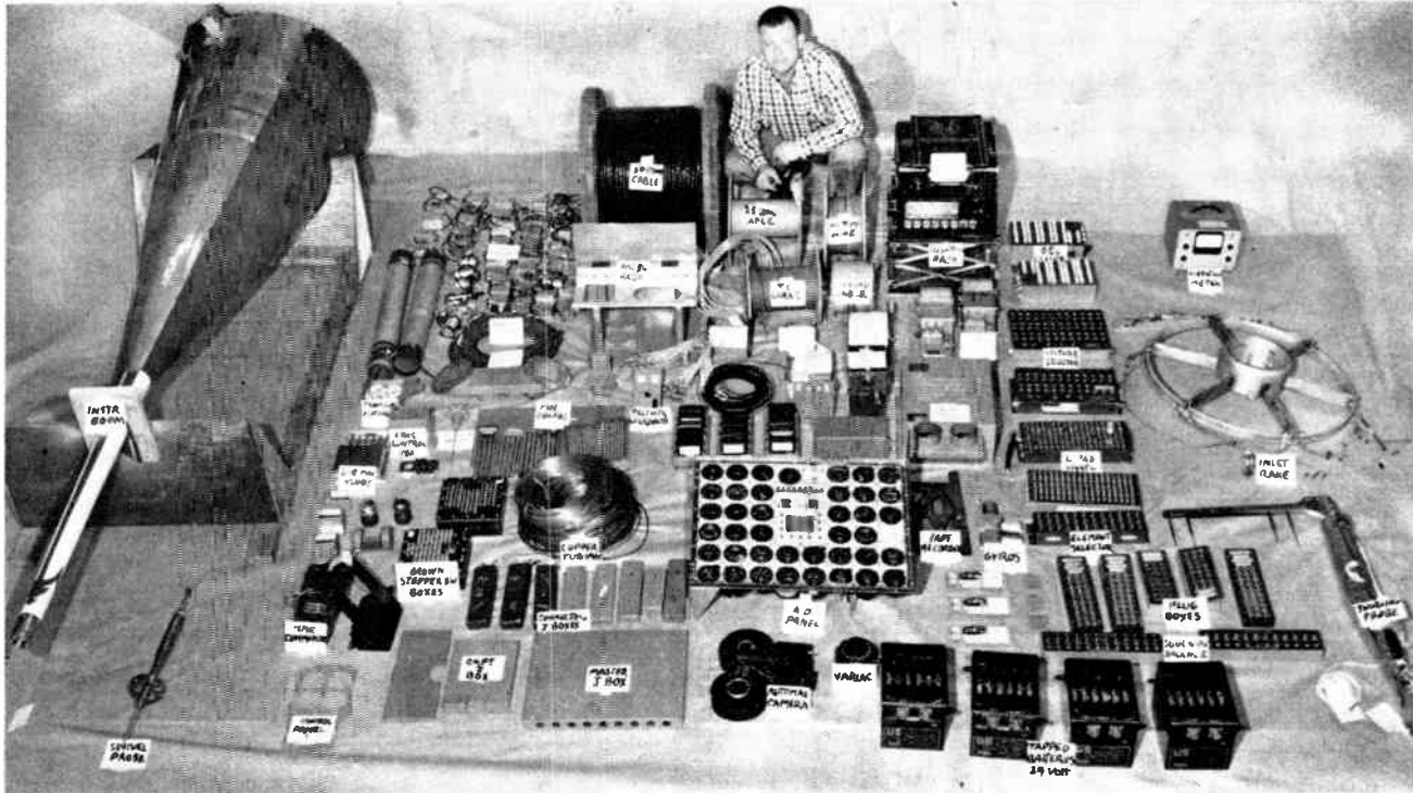
"Flight test package" for an average proving flight of the F-104 costs $200,000. Instrumentation for complex test flights may hit $1 million
