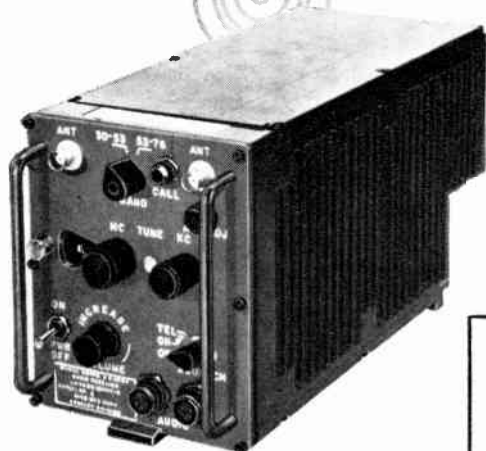
VHF, 920 Channels, fully transistorized Radio Receiver by Avco Mfg. Corp., Crasley Division
