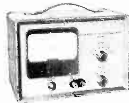
Ultra-Sensitive DC Microammeter WV-84B—popular choice for industrial, chemical and general laboratory applications. Designed to measure currents from 0.0002 to 1000 micro-amp. Can be used as ohmmeter to measure resistance in the order of billions of ohms. Self-contained batteries permit use for field applications. Low current drain tubes extend battery life; meter protected from accidental overloads. $110.00* (less batteries)
