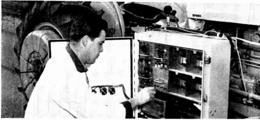
Proportional steering and start-stop signals provided by electronic system eliminate aching backs for tractor drivers on rugged test track
