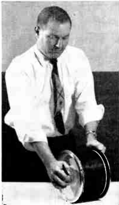
Engineer tightens connection on new transmit-receive tube for high power radar
