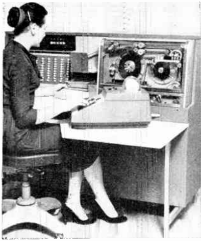
Assorted paper checks are magnetically-recorded at check-inscriber unit (left), only operation needed to ready them for automatic sorting, listing, etc., done by high-speed check-processing units (right)
