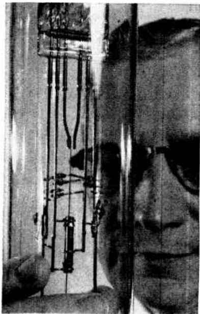
Wire emitter supplies electrons to collector through ionized gas
