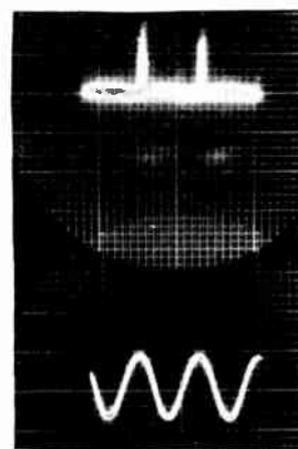
Contact resistance at 140 db sound-pressure level.
