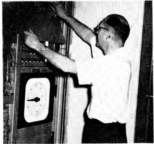
Scanning circuits feed analog-to-digital converter
