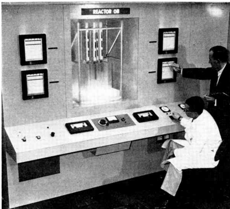
ELECTRONIC reactor simulator by Leeds and Northrup allows hazard-free training of nuclear reactor operators. Instruments behave just as they would on a real reactor. Student can watch model of reactor core while following operating procedure.
