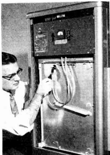
ELECTRONIC power supply delivers 13,000-v to grid of air cleaner
