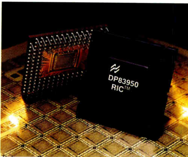
National's repeater-interface-control chip handles twisted-pair wire as well and thick and thin coaxial cable.
