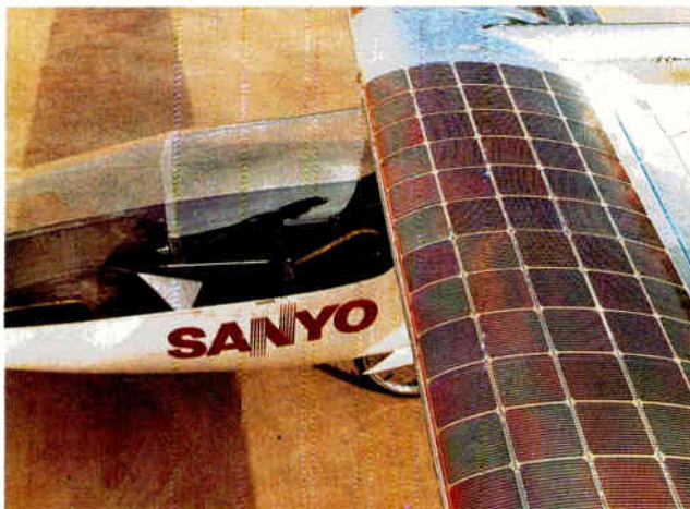
Arrayed on the wing of the ultralight aircraft SunSeeker are the Sanyo amorphous solar cells.
