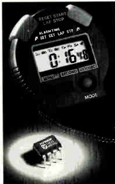
The low power PCF8583 provides a wide variety of timing functions.
