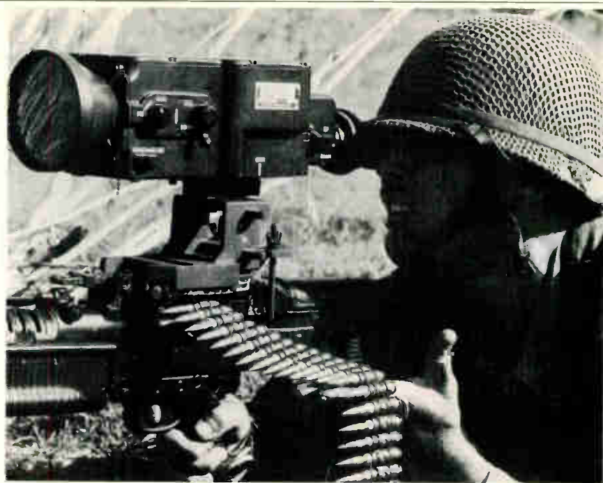
Focal-plane-array systems like this one, from Hughes Aircraft, let a foot soldier spot and track an enemy vehicle from several miles away.
