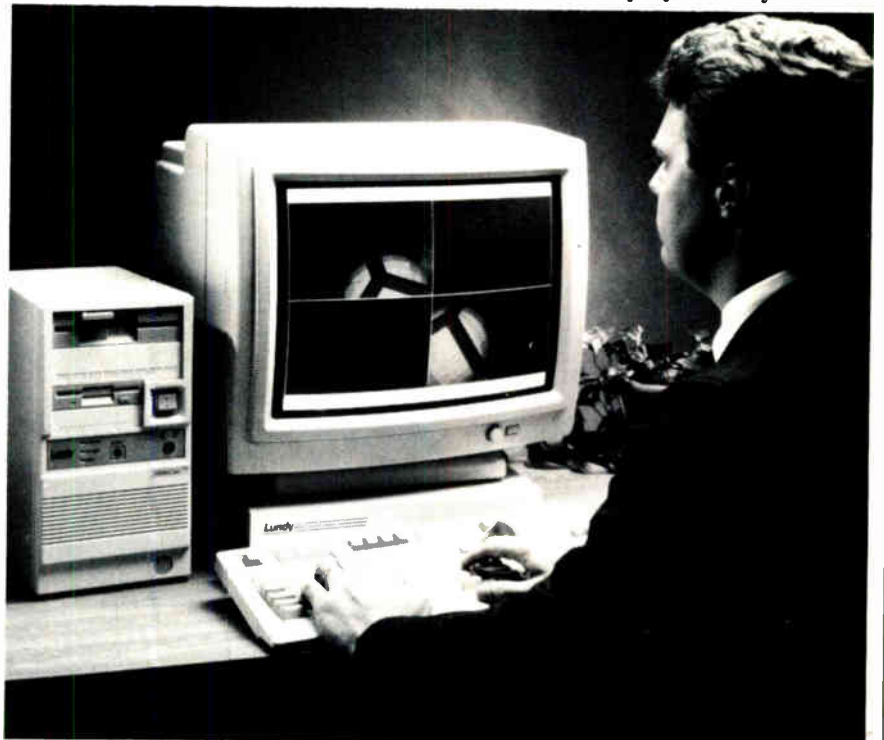
At the high end of the resolution scale is the Lundy 1612 Personal Graphics Workstation, which offers 1,600 by 1,200 pixels with 16 colors. It's based on the Texas Instruments 34010 processor.
