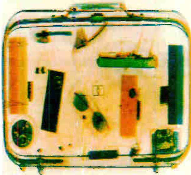
With color-enhanced X rays, plastic explosives appear orange while weapons are bright green.
