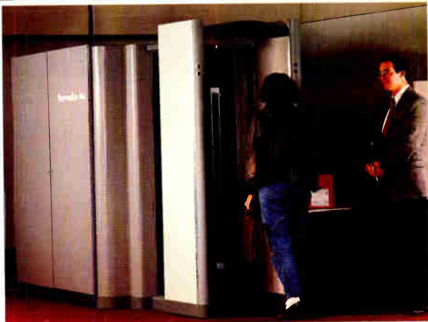
The Thermedics SecurScan system detects explosives by sweeping air around passengers and performing a chemical analysis.
