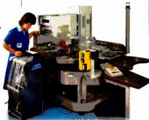
Surface mount 'Pick and Place' Machine, at AB's Microelectronics Plant.
