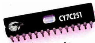
128K PROM 45ns, 100mA, 30mA Standby. 300 mil package. Three fast chip selects. Power-down chip enable. Reprogrammable. (Military: 55ns, 120mA, 35mA Standby.) Actual size!
