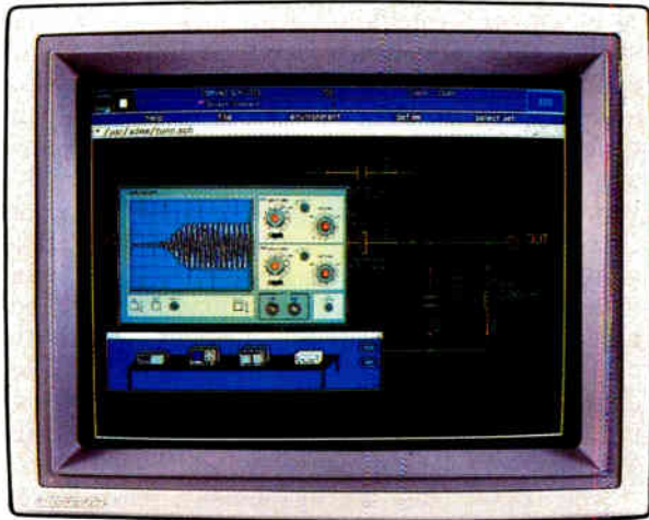
Easy-to-use virtual instruments provide a familiar interface for analog analysis using Intergraph's Cspice or ACS
