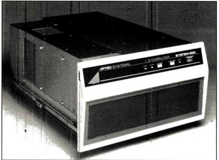
2. EXPANDABLE. The basic box contains one of each type of processor; more can be added as system I/O demands grow.
