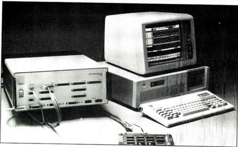
3. PARTNERS. The T100 analyzer can work with an IBM PC in a timing-analysis mode. Windows give user four views of recorded data.
