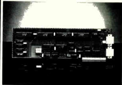
Model 1018-PC High-Density Parallel I/O Board used in Process Control, Automated Testing Equipment, Many Other Applications.
