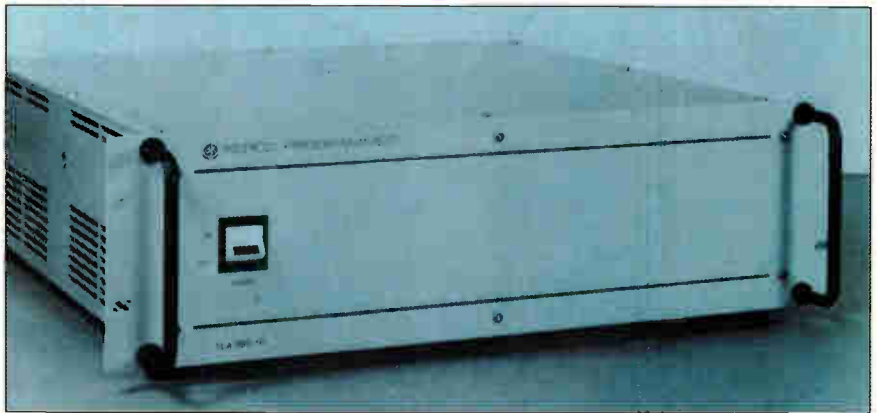
Kepeco's talker-listener device uses the high-level Control Interface Intermediate Language to communicate with up to 16 of the company's ATE Power Manager or BOP programmable power supplies at once. The parts are linked through an IEEE-488 bus.
