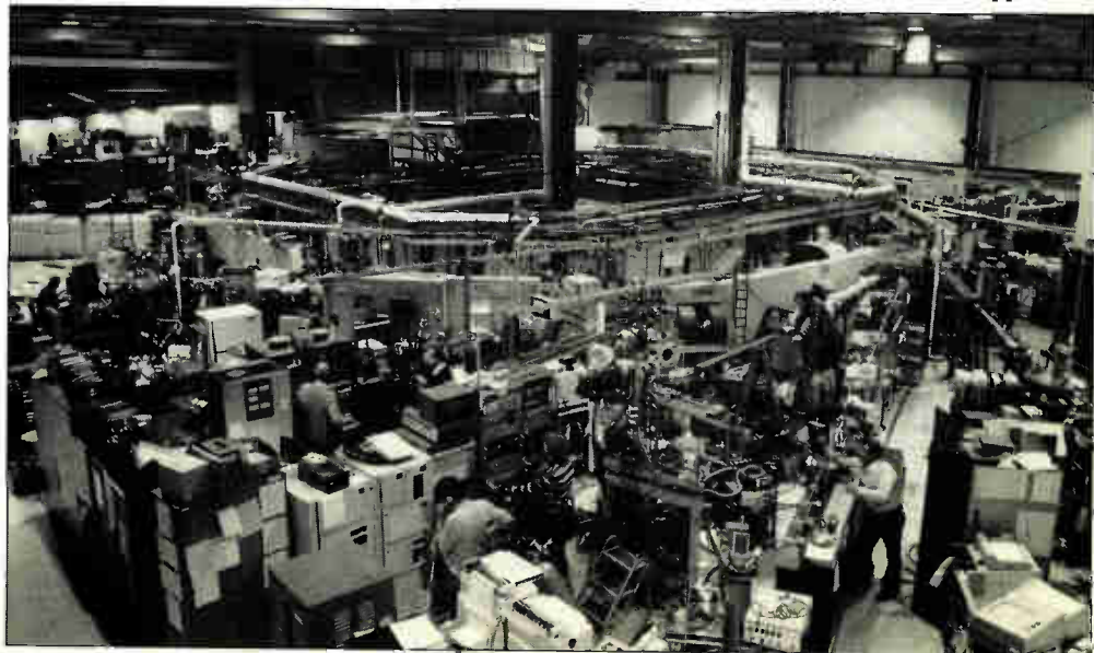
IN THE LAB. The vacuum ultraviolet synchrotron at Brookhaven spins off X rays for lithography.
