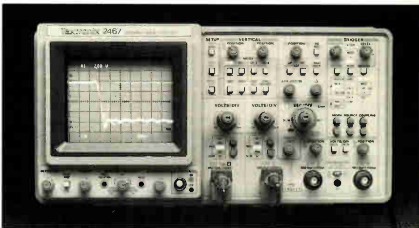
BRIGHT SPOT. A microchannel plate intensifies transients and makes them easy to spot.
