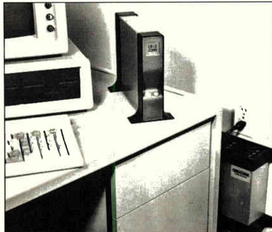
POWERLAN. A building's power lines provide the transmission medium for GridComm's 23-kb/s local-area network.
