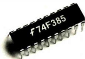
The new 74F385 quad serial adder/subtractor.
