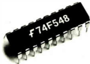
The 74F548 Octal Decoder/Demultiplexer
