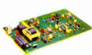
Remote Monitoring Equipment Modem
