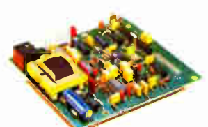
Data Acquisition Equipment Modem
