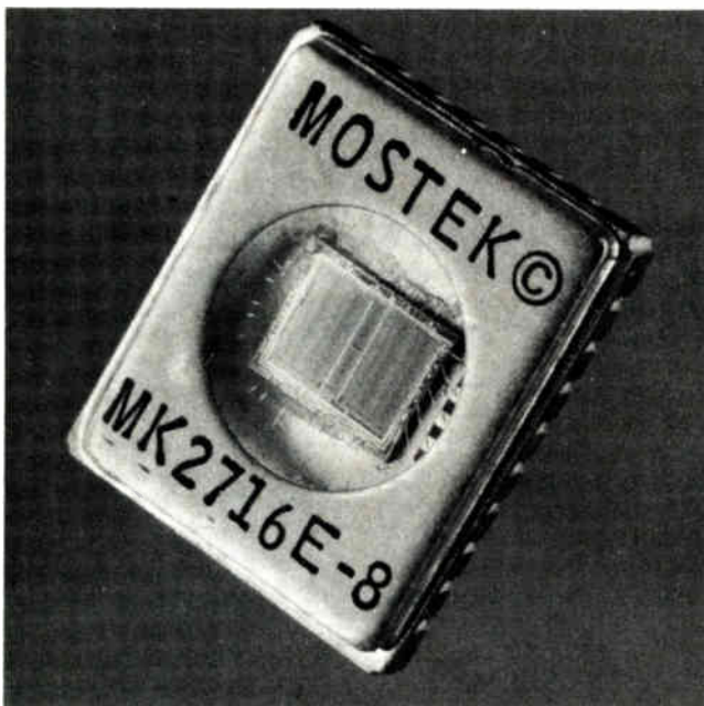
2. The right shape. Chip-carriers for memory chips are rectangular rather than square because of their elongated memory die within. The MKB 2716E 2-K-by-8-bit E-PROM is this view in a leadless type E package that measures 450 by 550 mils.
