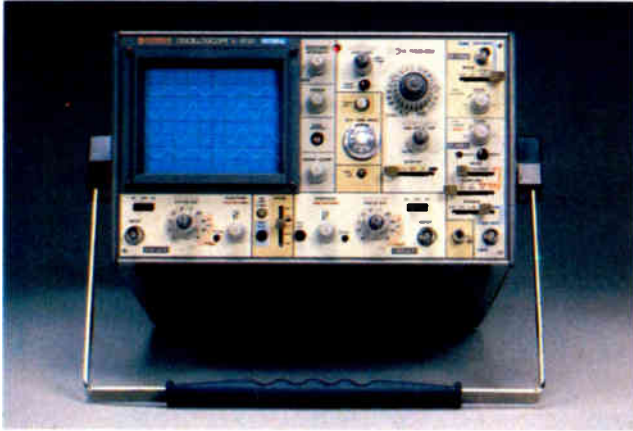
V-1050 100MHz QUAD-TRACE DELAYED SWEEP
