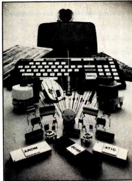
Products created for télématique will require a wide range of components, such as these RTC—La Radiotechnique Compélec parts for videotex terminals.
