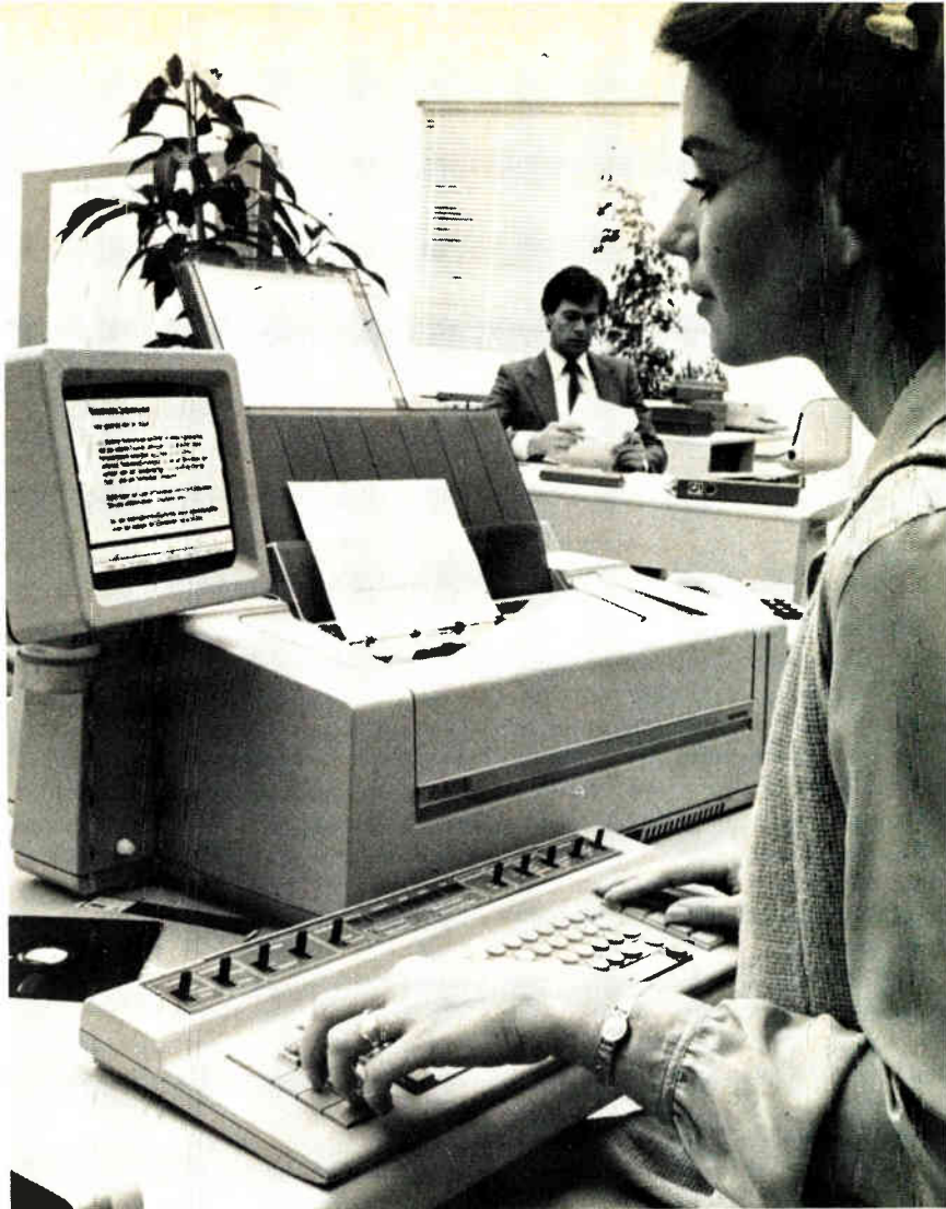
Sending the word. Electronic typewriters or word processors can be used for Teletex. This word processor from Siemens was developed specifically for the new technique.
