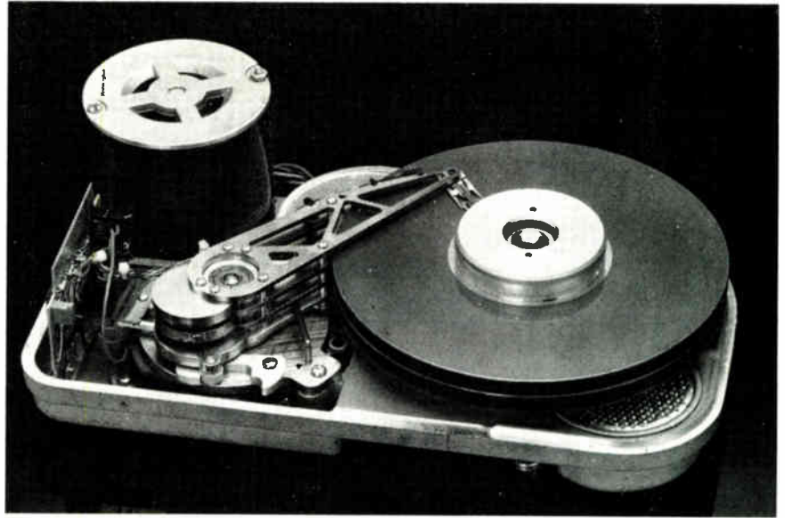
Denser. The Quantum Q2000 8-in. Winchester drive uses a novel actuator design and temperature-compensation method to achieve high densities at low cost.
