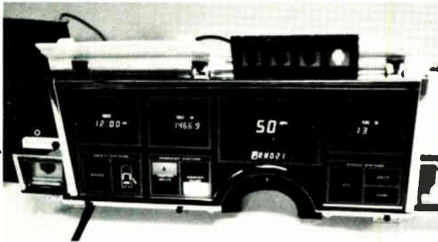
4. New look. Chrysler's new instrument cluster with electronic odometer is a standard feature on all 1981 Imperials. Vehicle speed, fuel supply, and even the gear selection indicator have gone to vacuum fluorescent blue displays for added appeal.
