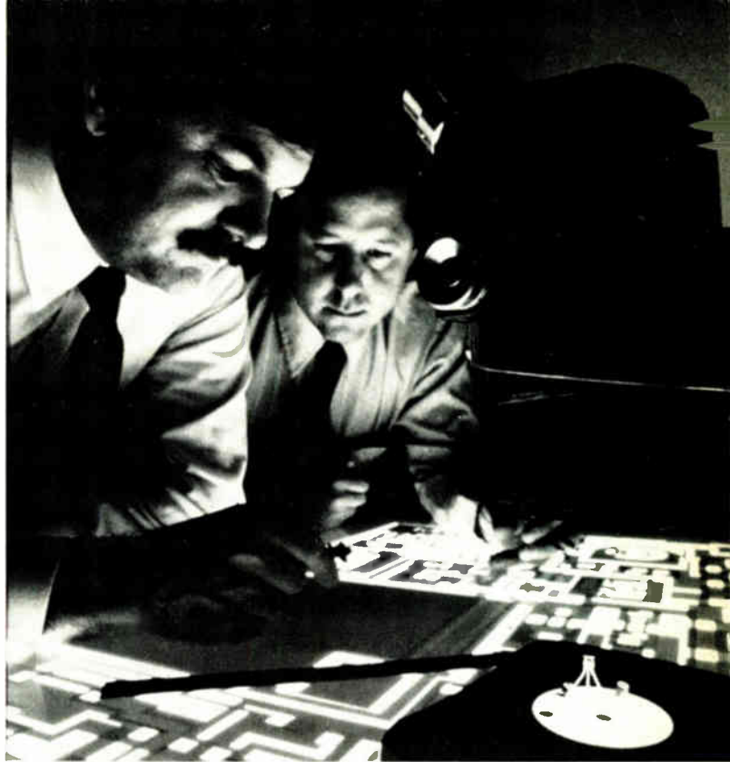
2. Lots of modules. TRW/Optron is preparing for the advent of monolithic fiber-optic receivers by developing a line of integrated devices. Here engineers Ben Wagner and Joel Van Antwerp check photo mask artwork for accuracy on a light table.
