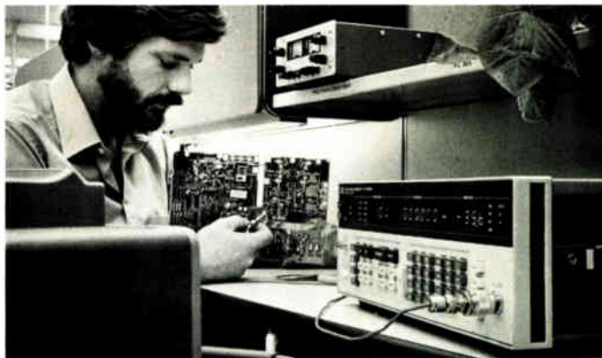
HP-IB programming is standard in HP's new 8656A Signal Generator. In that mode, frequency switches in less than two seconds (to be within 100 Hz).
