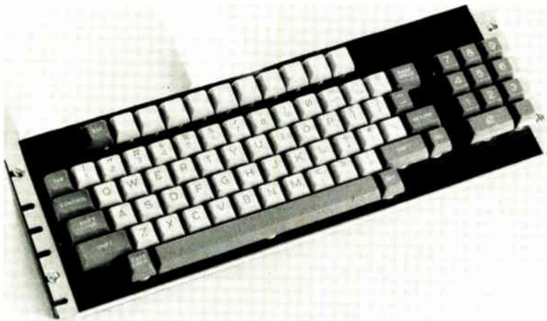
Back to keys. Although membrane-switch technology lends itself to flat keyboards, for data-entry applications, it is being combined with raised keys because users prefer them.
