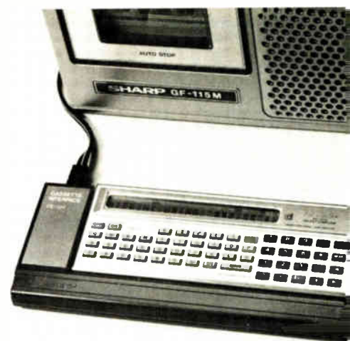
Out of pocket. Sharp's PC-1210 pocket computer is shown linked to cassette player via its CE-121 cassette interface device.
