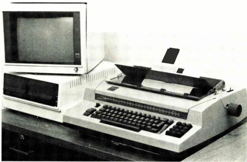
Easy fit. A standard desk extension will hold the new Aquarius word processor, which employs the electronic version of the IBM Selectric typewriter as keyboard and printer.
