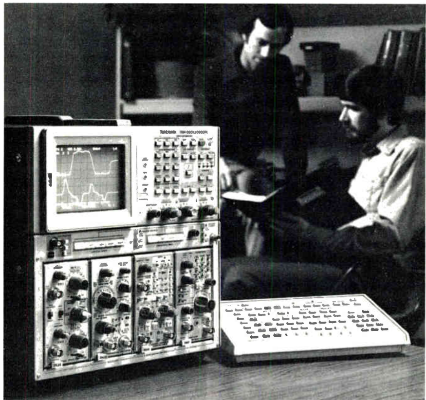
Combination. Tektronix' new digital storage scope incorporates a 16-bit microprocessor to process waveforms and perform measurements and computations at the touch of a button.
