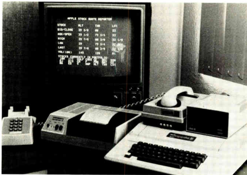
Market aid. Apple's Stock Quote Reporter shows current prices, permits bid to be made, ascertains closing price, high and low price for the day, and current volume of a stock.
