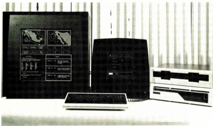
Big picture. Largest ac plasma panel has 24-in.-diagonal picture and can display over 21,000 characters. It was developed by Photonics Technology with Science Applications Inc.
