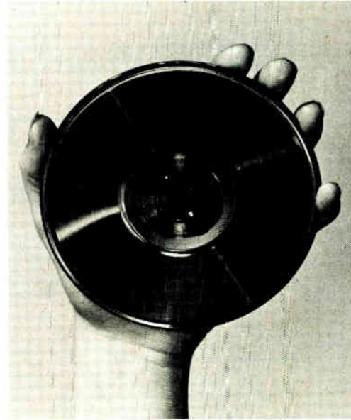
For the record. Proposed PCM audio disk from AEG-Telefunken and Teldec is 13.5 centimeters in diameter and comes housed in a protective cassette (not shown).
