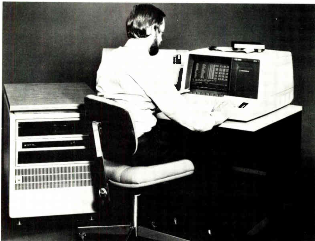
Universal. Hewlett-Packard's first microprocessor development system will support numerous processors and as many as six development stations. It has hard-disk storage.
