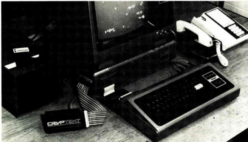
Secret stuff. By plugging in the Cryptext encryptor-decryptor, users of TRS-80 small computers can turn data into scrambled patterns. Units for similar computers are next.
