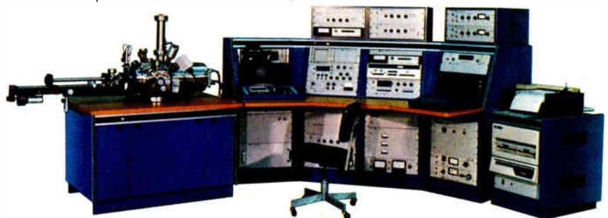
Three-dimensional materials characterization using Auger analysis with ion sputter-etching.
