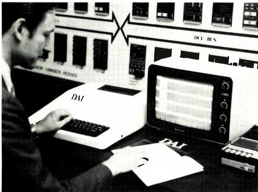
Homeward bound. DAI's personal computer has up to 22 kilobytes of ROM and up to 48 kilobytes of program RAM, together with a range of input/output devices.
