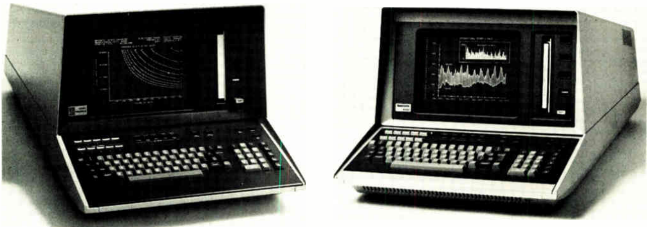
Fraternal twins. Although the units are nearly identical externally, the processor in the 4052 is totally redesigned, replacing the 4051's 6800 with a bit-slice emulation. As a result, the former is much faster than the latter yet retains software compatibility.
