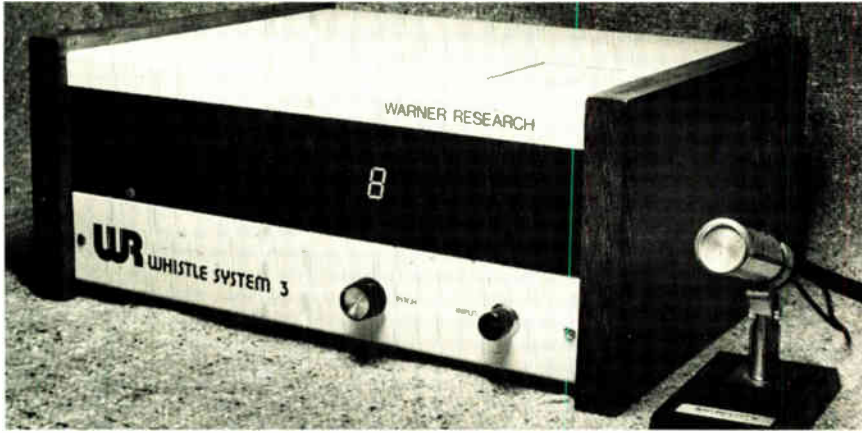
Helper. Electronic aid for the handicapped senses a whistle signal, then activates the appliance corresponding to the number shown on the unit's light-emitting-diode display.
