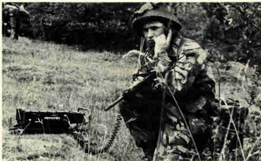
Single-channel. Plessey's new Groundsat repeater unit, shown in simulated army maneuvers, permits a vhf mobile system to operate easily over distances on a single frequency.
