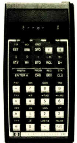
HP-33E, Programmable Scientific. 49 program lines of fully merged key codes. Editing, control, and full range conditional keys, plus 8 user memories.
