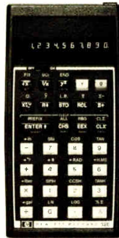
HP-32E, Advanced Scientific with Statistics. More math and metric capabilities than HP-31E, plus 15 user memories, hyperbolics, comprehensive statistics.
