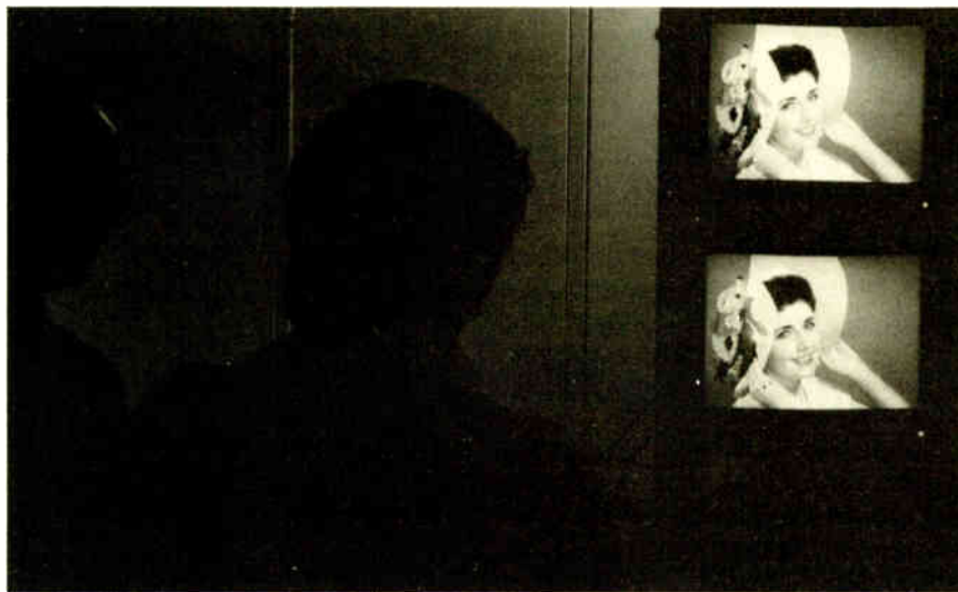
Good show. Sending a test TV picture on a 70,000-km round trip to a satellite hardly affected quality when SEL used its experimental 34-Mb/s equipment with a 10^{-9} bit-error rate.
