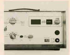
Semiautomatic attenuation tester DT-1 feeds a 1-kHz sine-wave noise signal into the line and then measures noise level with its built-in level meter. Automatic range selection of results simplifies operation. Felten & Guilleaume, 5 Cologne 80, P. O. Box 805001, West Germany [460]
