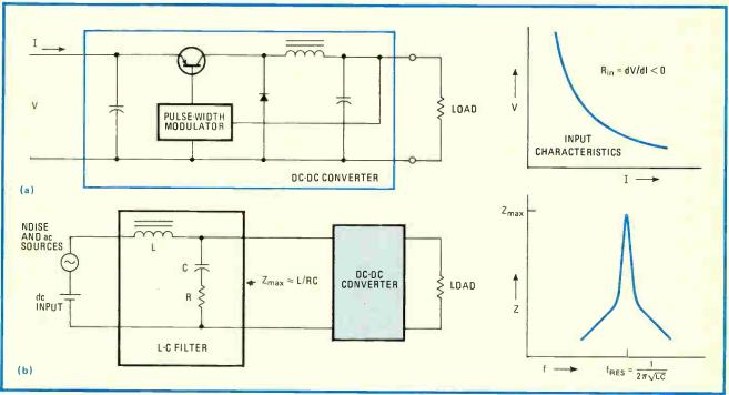
Filter interaction. Switching dc-dc converter (a) exhibits negative input impedance, causes converter/noise-filter combination (b) to oscillate at  $f_{res}$  if  $Z_{max} > R_{in}$ . For proper filtering, and to eliminate the possibility of oscillations, filter's L-to-C ratio must be reduced.
