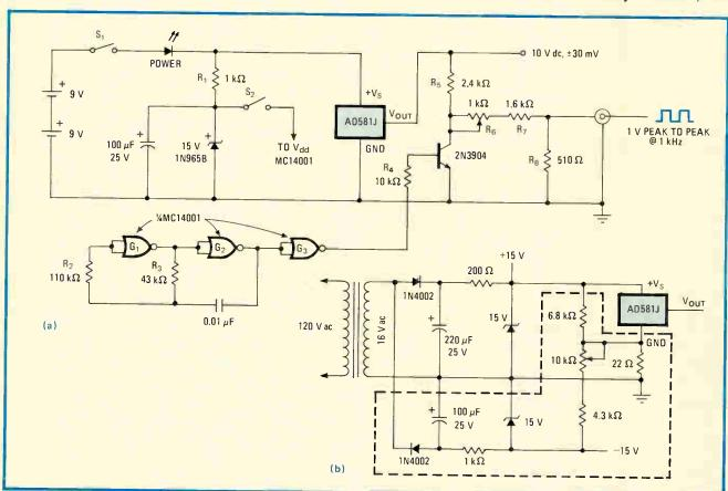
**Precise amplitude.** Scope calibrator generates 1-V square wave, accurate to within 0.5%, with aid of AD581J band-gap voltage reference (a). Unit may be powered by two 9-V batteries. Current drain is 6 mA. Ten-volt reference voltage is available at output jack for voltmeter calibration, etc. If more than occasional use is contemplated, the unit should be powered from the ac mains (b).
