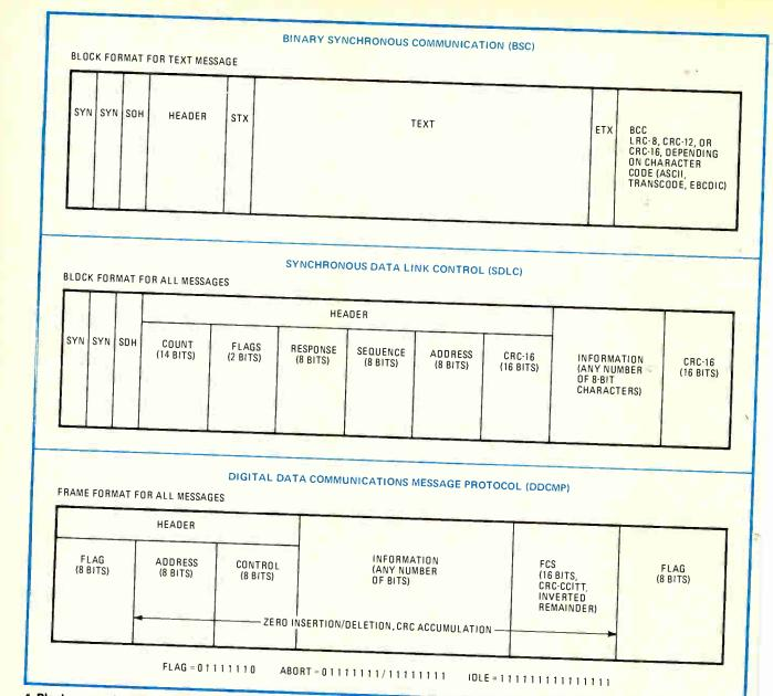
4. Block comparisons. The three different protocol schemes generate three different block formats. IBM's Bisync uses a character-controlled arrangement; DEC's DDCMP relies on a character-count procedure; and IBM's SDLC employs a bit-oriented protocol.
