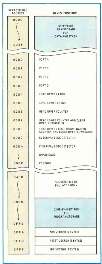
2. Address selection. The efficient addressing in the 6500/1 has random-access memory occupying the first 64 locations. Together with I/O, RAM is on page zero—the first 256 bytes—which can be addressed with a single instruction. There are 13 address modes.
