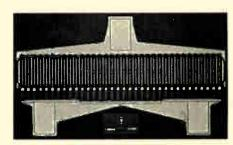
Internal matching at input enables broad bandwidth designs with this 34-finger ballasted transistor.
