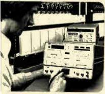
wlett-Packard's new 3771A performs troubhooting measurements to CCITT standards high speed data transmission lines. When ed with the existing HP 3770B Telephone e Analyzer, shown in background, they proe a complete, portable data line test system.
