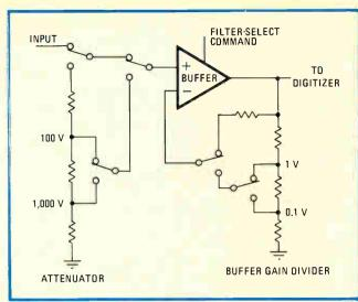
4. Stable elements. The accuracy of the 6000 depends on the design of the input attenuator and the stability of the isolating buffer amplifier, which also contains a selectable filter to combat noise.
