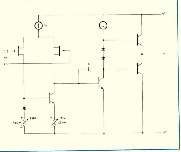
4. Low cost. Bi-FET op amps that are less complex and expensive than the LF356 are made by using laser trimming to adjust offset voltage right on the chip, instead of optimizing the design for low offset as with the LF356. A zener and a resistor set the input bias current.
