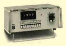
The type 300 digital ohmmeter can measure from  $10\mu\Omega$  to 20 M $\Omega$  in 13 decades. Use of a four-wire technique reduces the maximum error to 0.1%. All leads are shielded to reduce risk of false measurements. Dietechnik, 8041 Weng, Am Kirchfeld 2, West Germany [456]
