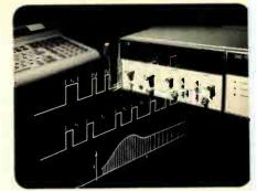
HP's 5391A Data Acquisition System is capable of over 50,000 measurements per second in frequency, period, time interval, ratio, or totalize mode.
