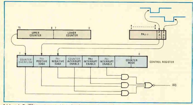
5. Interrupts. The IRQ interrupt request originates from three sources that are each software-maskable: the rising edge at pin PA<sub>0</sub>, the falling edge at PA<sub>1</sub>, and counter overflow. The other interrupt, NMI, is non-maskable and is used for critical events such as power failure.
