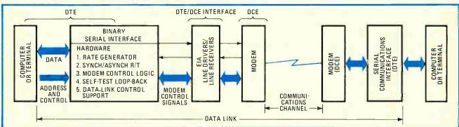
1. Linkage. Modems, serial communications interface, and communications channel are all part of basic data-communications link. Data-link controls are needed only for the link, not for the computer or its peripherals. The modem can also be a data-service unit for Dataphone digita service, a line driver and line receiver (modem eliminator), or an interface with a satellite or microwave channel.
