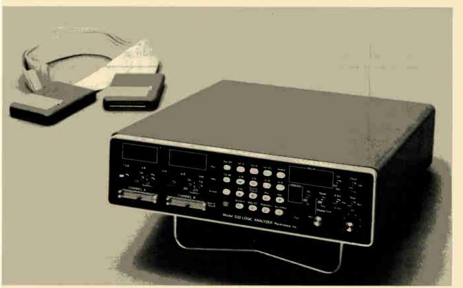
Fast service. Combining the best of two analyzer worlds, the model 532 captures 250 32-bit words of logic-state data and automatically computes and displays two associated signatures that identify faults in the microprocessor-based system under test.
