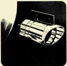
IRAS - Infra-Red Astronomical Satellite-due to be launched into a 900 kilometre polar orbit in 1981, is the first scientific satellite designed to make a detailed inventory of infra-red sources in space. The on-board computer, which will process about 500 million bits of measured data per day, will be supplied by us along with other electronic systems.
