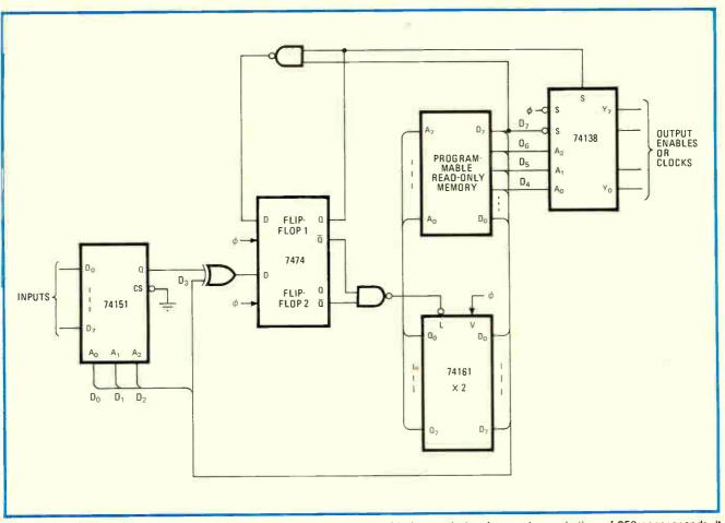
6. Sending data. The algorithmic state machine, a 256-word-by-8-bit variable-format design, has a microcycle time of 250 nanoseconds. It executes two types of microinstructions: store output and conditional jump, taking one and two microcycles, respectively.
