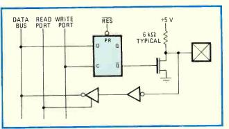
3. No direction. The bidirectional input/output lines require no direction register. Normally written to 1, an input is overridden by a 0, which latches the D-type flip-flop driving the transistor low. The 6-kilohm pull-up resistor can be omitted with a mask option.
