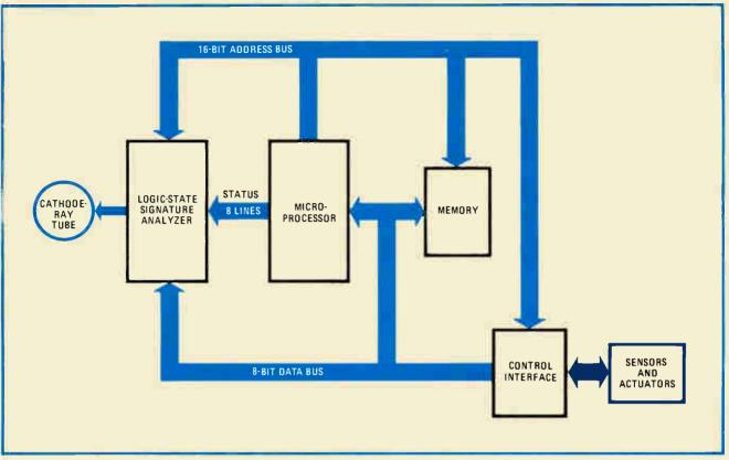
4. Checking a controller. In monitoring the performance of a microprocessor-based industrial controller, the 532 is first used with the product operating under laboratory conditions. Then it looks for signature changes as the environmental conditions are varied.
