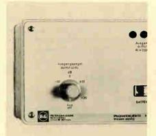
Speech-noise generator model RGS-1, for speech simulation on telephone channels. produces a quasi-random noise signal using MOS shift registers. An active RC filter performs a spectral evaluation. Felten & Guilleaume, 5 Cologne 80, P. O. Box 805001, West Germany [452]
