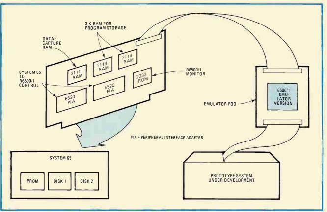
**6. System design.** With the 64-pin prototyping version of the 6500/1 on an emulator board, external memory can be used in lieu of the chip's built-in memory. The memory board has a read-only-memory monitor that adapts the 6500/1 to the System 65 for development.
