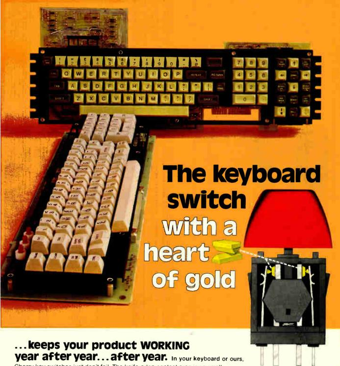
Cherry key switches just don't fail. The knife-edge contact area is so small (9 millionths of a square inch)... the contact pressure so great (about 5,000 psi)... the gold alloy so pure and film-free... that you are assured of positive contact every time. For 50 million operations and beyond. (Which is probably beyond the life expectancy of your product!)
