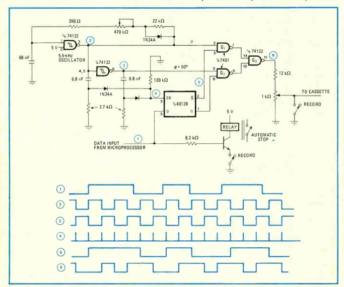
1. Inexpensive. Low-cost microprocessor-to-cassette interface can be used with tape recorder to form economical data-storage system.
