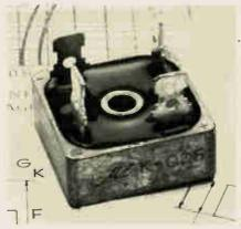
Single-phase full-wave bridge rectifiers, designated the J and K series, are meant for use in high-current applications—up to 10 A and 25 A maximum average dc output current, respectively. Micro Electronics Ltd., York House, Empire Way, Wembley, Middlesex, England [447]
