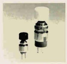
The 9100 momentary push button is 6.5 mm in diameter and 17.5 mm in overall length. Its contact resistance is less than 30 m $\Omega$  and its insulation resistance is greater than 1,000 M $\Omega$  measured at 500 V. It has a life of 300,000 operations. APEM, B. P. 1, 82300 Caussade, France [450]
