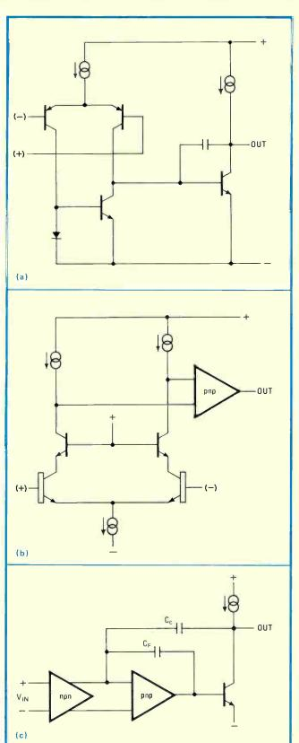
2. Evolution. Monolithic bipolar op amps have proliferated because of the evolution of circuit innovations. For example, the 709 (a) incorporates lateral pnp transistors to solve dc level-shifting problems, the 108 (b) has superbeta npn transistors for better input characteristics, and the 118 (c) uses a feedforward technique to improve bandwidth and slew rate.
