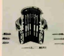
Voluminous filter sets are replaced by these pin contacts with integrated filters. The contacts handle up to 5 A and are available with  $\pi$ , C, LRC, and CLR characteristics. Connectors house from 3 to 64 contacts. Amphenol-Tuchel GmbH, 8024 Oberhaching, West Germany [457]
