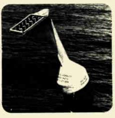
Solar energy is used to re-charge the storage battery aboard each of the forty survey buoys currently performing a marine study in the Indian Ocean. Continuously monitored data is automatically transmitted from each buoy every hundred minutes via the Nimbus-Six satellite. The study is being carried out by the Commonwealth Scientific and Industrial Research Organisation (CSIRO). Philips supplied the solar collector panels.
