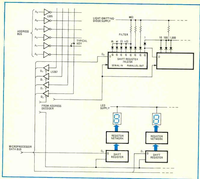
1. Slow but sure. Because much of the formatting, conversion and coding is done in software, the display/keyboard hardware in the 6000 comprises relatively few parts. Although execution is relatively slow, there is a net gain in versatility.
