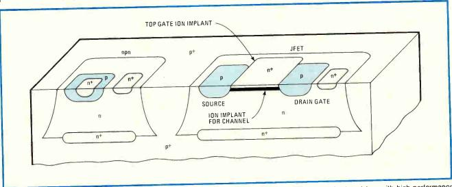
1. Basic structure. Because of ion implantation, bi-FET circuits can combine high-performance bipolar transistors with high-performance matched JFETs. One implant creates the p channel between source and drain contacts, another the gate region over this channel.
