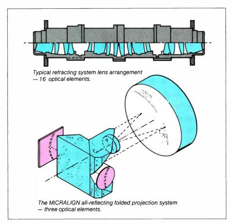
Compare these two lens systems. Until Perkin-Elmer introduced the Micralign Projection Mask Alignment System five years ago, all manufacturers of projection systems used refracting optics. Most still do.
