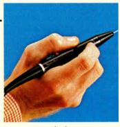
matically compares logic traces with the recorded reference traces. Pass-Fail lights on DTO-1's probe guide technicians through complete testing of product functions. You get improved quality control. It's quick and it's foolproof.
