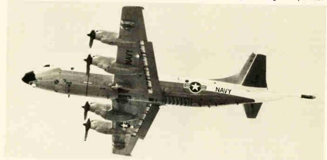
**Sub chaser.** The P-3C Update II Orion land-based subhunter incorporates a variety of new sensors, avionics, and weapons. Included are a passive infrared-detection system and the Harpoon antiship missile that enables the aircraft to attack surface targets 60 miles away.
