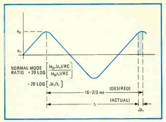
3. Normal-mode rejection. If the integration period is not identical to the power-line period, the system's rejection of power-line noise is adversely affected. An internal oscillator controls the integration period to ±.01%, essentially limiting normal-mode rejection to 48 dB with the expected 60-cycle line variations.
