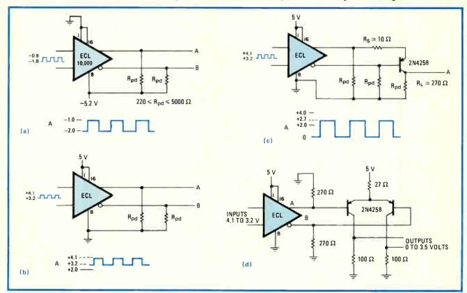
Evolution of an interface. Standard emitter-coupled logic is powered by at least one negative voltage, cannot drive or be driven by TTL (a). Re-biased ECL device generates positive output voltage, but not within proper TTL switching threshold range (b). Adding a transistor enables 0-2.7-V swing, suitable for TTL (c). Five-volt ECL gate and two transistors drive 100-ohm TTL loads at 0-3.5 V (d).
