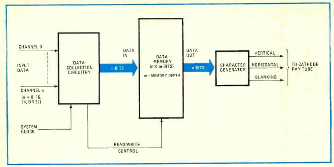
1. Localizing faults. In the basic logic-state analyzer, parallel data is clocked synchronously into a memory for later display in binary. hexadecimal, or octal notation. The instruments are widely used in monitoring sequential machine states and in software debugging.
