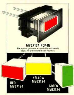
You're assured of uniform illumination across a large emitting area (.15" x .25"). This new package makes maximum use of emitted light, minimizing unusable light. Light output is a very bright 4 millicandelas at 20 mA (red and yellow) and 3 mcd for green. That's up to 3 times the output of other rectangular lamps.
