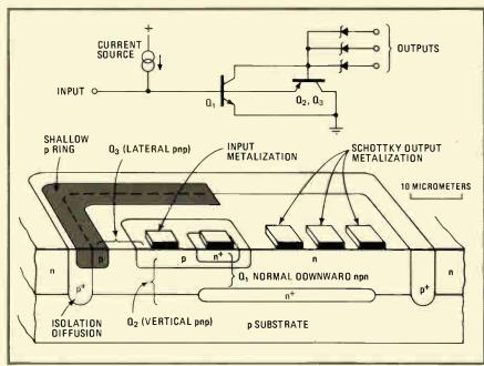
**New logic.** In ISL, the normal downward npn transistor inherently adds a vertical pnp device. A p ring parallels the vertical transistor with a lateral pnp one.
