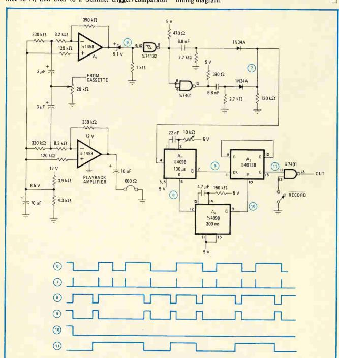
2. Retrieved. Data is recovered after passing through receiver interface using process essentially inverse to one used at transmitter. One-shot A₂ is used to convert input signal to two complementary 130-μs waveshapes. One waveform drives a second one-shot, A₄, which in turn resets A₃, while the other waveform drives its clock input. Timing diagram details operation. Output is a delayed version of the original signal.
