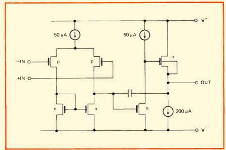
On a chip. In experimental LSI operational amplifier built with complementary-MOS technology, dc gain is 90 dB, slew rate is 2.5 V/µs, and common-mode rejection is 65 dB.
