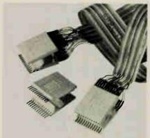
The series PC14 to PC40 test clip adapters connect to integrated circuits with from 14 to 40 pins for applying power to them and performing functional tests. The chance of short circuits is eliminated. Atlantik Elektronik GmbH, 8 Munich 70, Hofmannstr. 20, West Germany [459]
