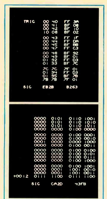
3. Identifying data. The data in the model 532 main memory can be displayed in the form of 16-word pages on a scope in hexadecimal (top) or binary (bottom), along with the identifying signatures.
