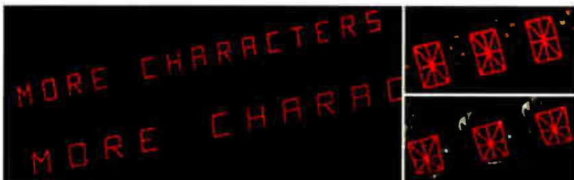
Left: More characters—MAN2815 (top) and competitive unit character density in same panel space. Right: Less distortion—MAN2815 (top) and competitive unit when viewed 25° off of normal.
