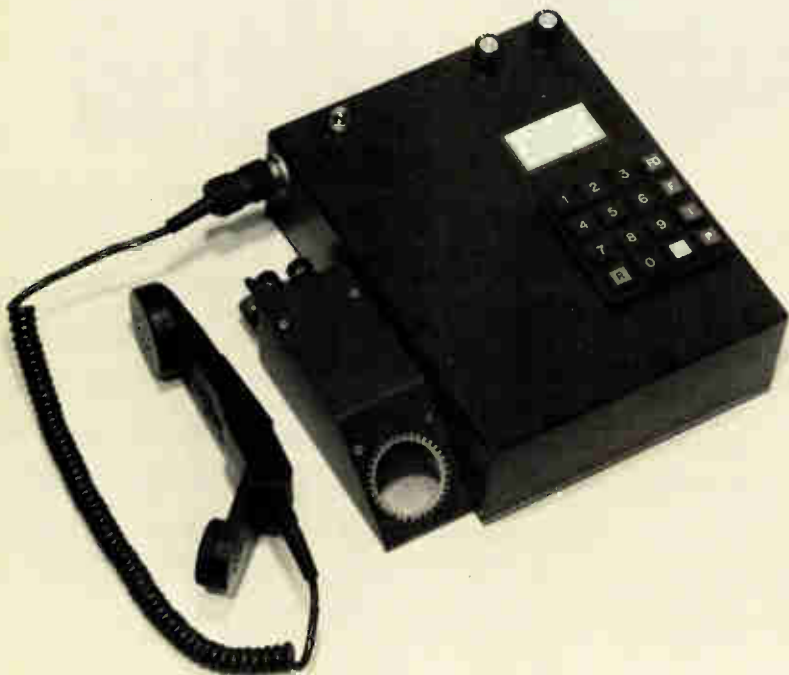
Digital. Electronic Communication Inc. has delivered 25 digital telephones to the Air Force for the Tri-Tac system. Phone's three main sections are on three circuit boards.
