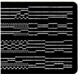
Time Domain. Timing diagram you see the sequential and simultaneous relationship between digital signals, to simplify hardware troubleshooting.
