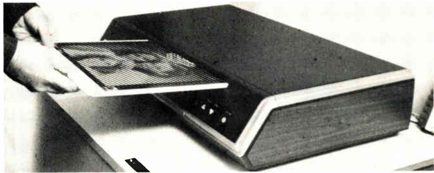
Player. Protective polystyrene permanently covers VideoDisc, shown being inserted in demonstration player. Disk material holds shape to 135°F, RCA says.
