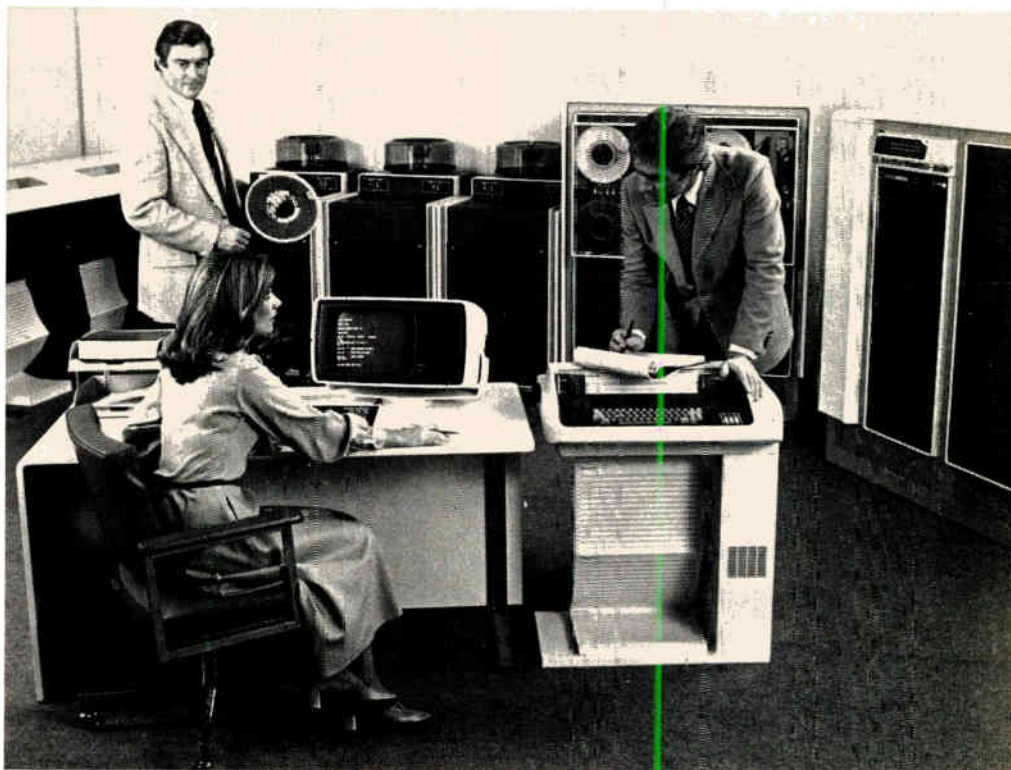
Host. Eclipse M/600 system could play host in a distributor's inventory management net. Price of $325,000 includes computer, 512 kilobytes of main storage, tape and disk drives, display and printer consoles, and 48 local and remote time-sharing terminals.
