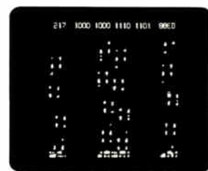
Map Mode. Each digital word can be translated into a singularly positioned dot in this graphic representation of recorded data. Especially useful for spotting illogical or illegal memory addresses.
