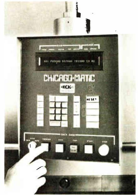
Entry point. Most of the press brake's setup and control is handled through this microprocessor-based control console.
