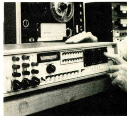
Cleaner. Rockwell's automatic digital audio processor eliminates unwanted noise from audio signals and recordings in real time.
