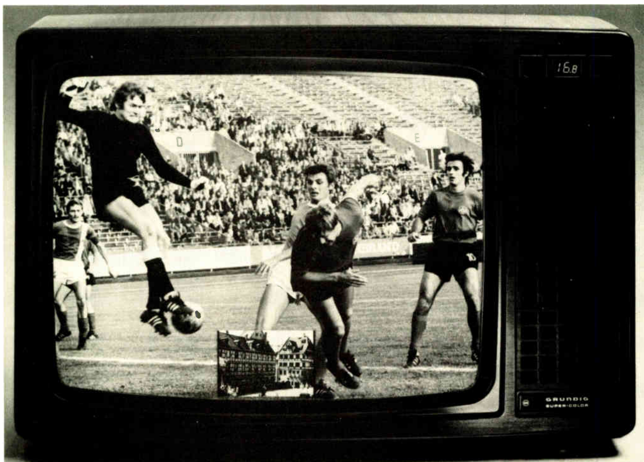
1. Picture in a picture. Grundig's 26-in.-diagonal color TV set is able to display simultaneously with the main picture a small, 4.5-in.-by-3-in. black-and-white inset from another channel, thanks to circuitry on a special small chassis built into the large set.
