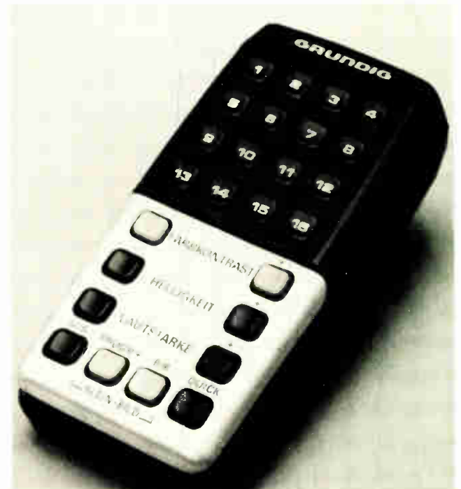
5. Double selector. Grundig's IR remote-control transmitter can select as many as 16 large picture and eight inset picture channels. The viewer may select only the large picture or may shift back and forth between the large and small pictures.
