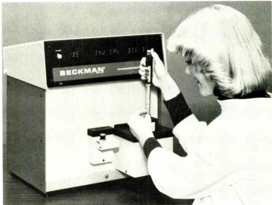
Twin functions. Gas-discharge display on the immunochemistry analyzer can be turned into the display for a digital voltmeter when faults must be located in the equipment.
