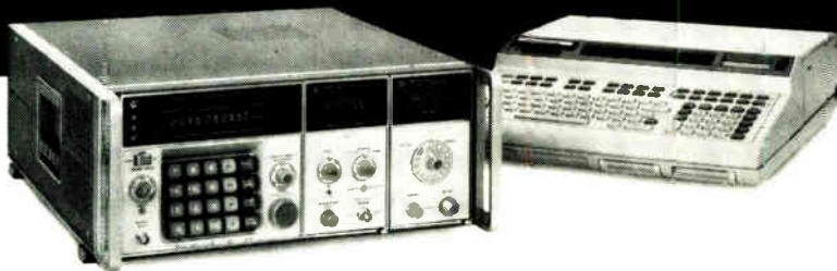
3. 8660C Synthesized Signal Generator under 9825A Desk Top Computer Control provides fully programmed signals from 10 kHz to 2600 MHz with AM, FM, phase or pulse modulation.
