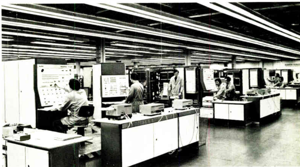
Checking it out. At VEB Robotron-Elektronik in Dresden, EC2640 central processing units undergo tests. East Germany's computers mesh with those of others in Comecon.
