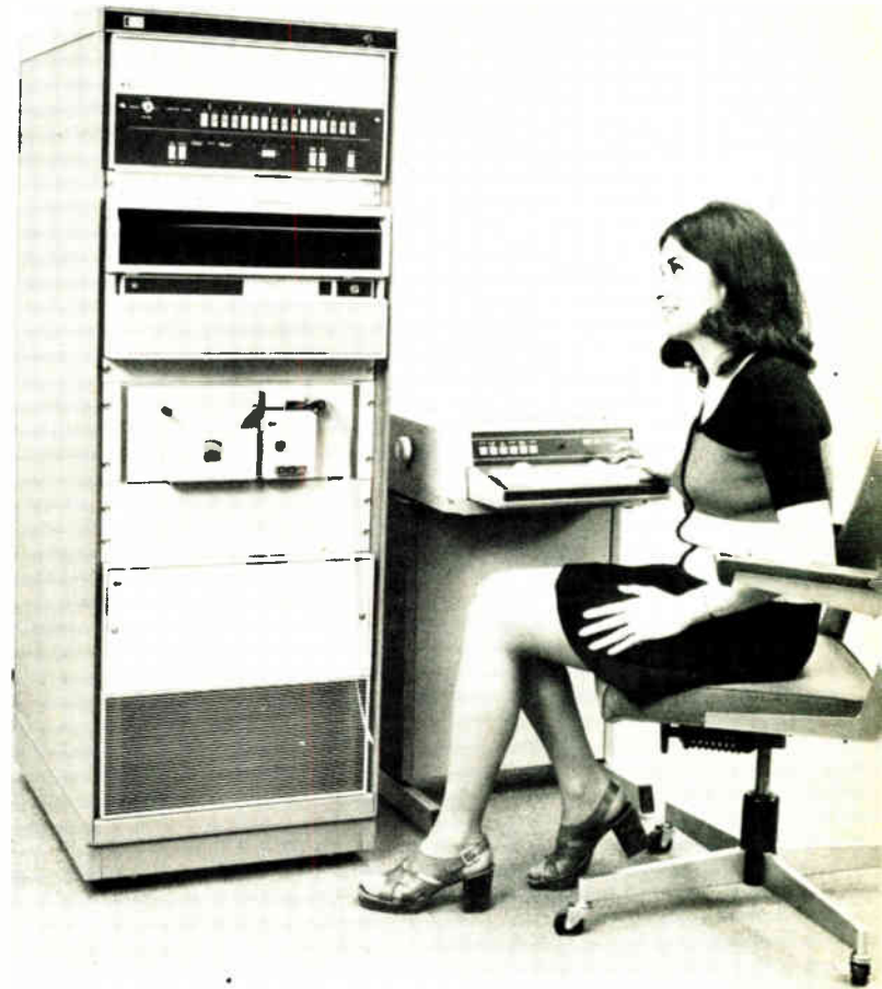
Large. Beefed-up cousin, the H-P 2108A, appears here at the top of the rack in a typical disk-based system. It has a 32k-word memory and nine I/O channels. Both machines are among the first large-scale applications of 4,096-bit MOS memories.
