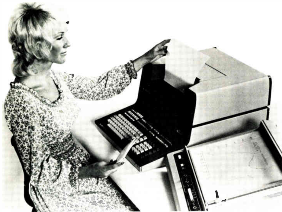
The programmable calculator's capabilities are extended with such added peripherals as the 9862 graphic plotter.
