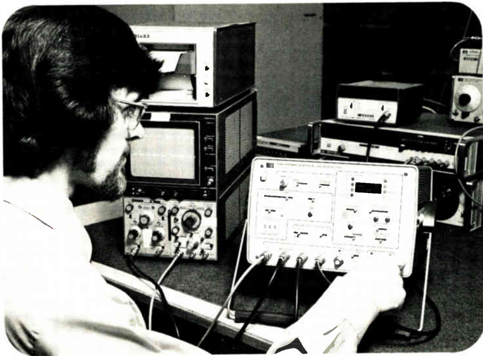
The 3780A Pattern Generator/Error Detector is a complete 1 kb/s to 50 Mb/s error measuring set in one portable package.
