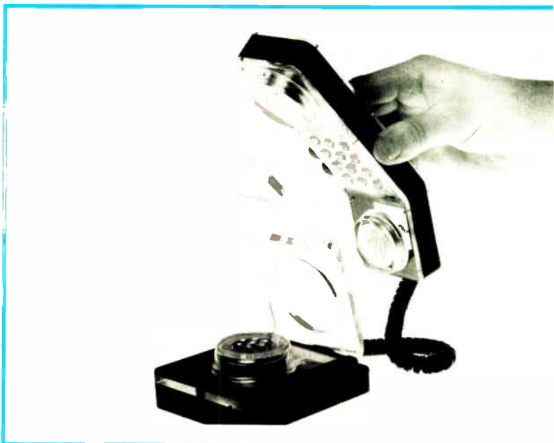
1. First of a kind. Bell Northern Research has developed an all-electronic telephone using LSI circuitry to replace the electromechanical parts of conventional telephones. One result is that future phones could take many shapes, as the model shown suggests.
