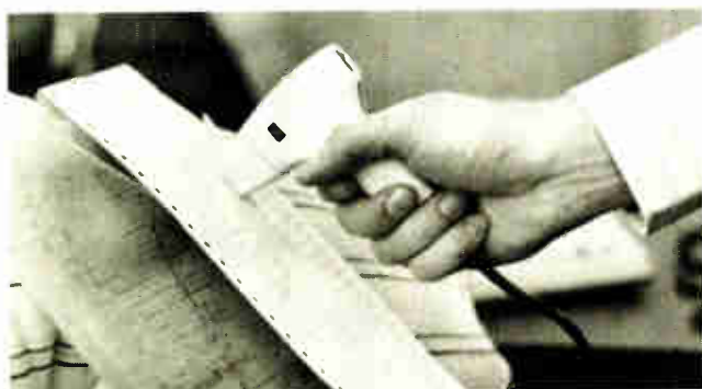
5. Optical magic. The Key Tronic OCR wand (top) uses a wheel moving across the paper to generate pulses that cause the photodiode array to take readings every 1/200 in., while the Recognition Products wand need not be in contact with the paper.
