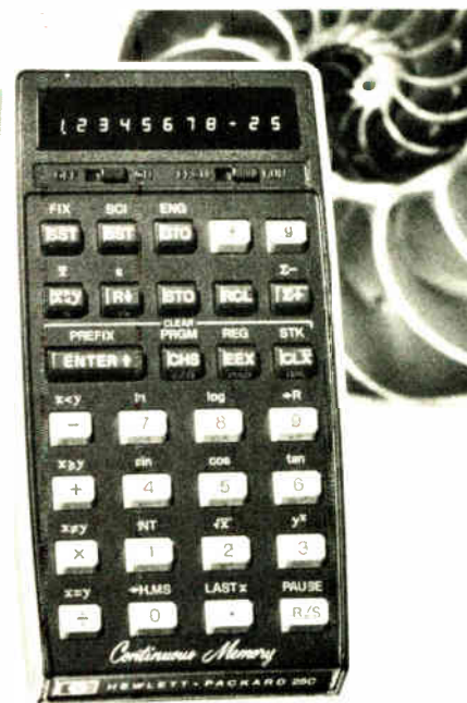
2. Watch memories. Microma's LCD chronograph watch (left), which sells for under $100, is based on a mask-programable MOS circuit from Intel. Hewlett Packard's HP-25C programmable scientific calculator has a C-MOS continuous memory that retains input when turned off.
