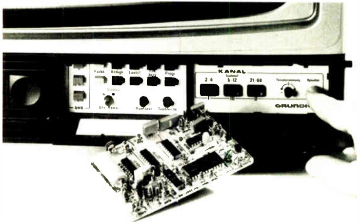
1. Selection. All-electronic tuning has been advancing rapidly in West Germany. For example, this Grundig channel-selection system designed jointly with TI, features scan and select frequency search. When user finds correct frequency, he enters it into memory.
