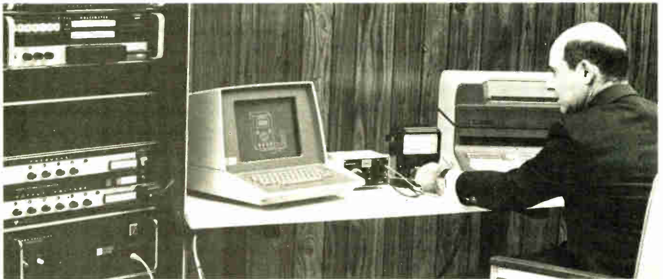
3. Calculator control. As the speed and flexibility of desktop programmable calculators increase, more of these devices are applied in automatic test systems such as this Julie Research calibration console. The tester can generate images of the unit under test on a graphics terminal, thereby simplifying the location of test points and controls.
