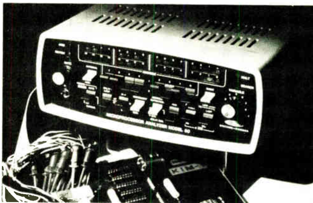
1. Microprocessor monitor. Analyzers like this Systron-Donner unit simplify microprocessor-program generation and debugging by displaying the activity on address and data buses.
