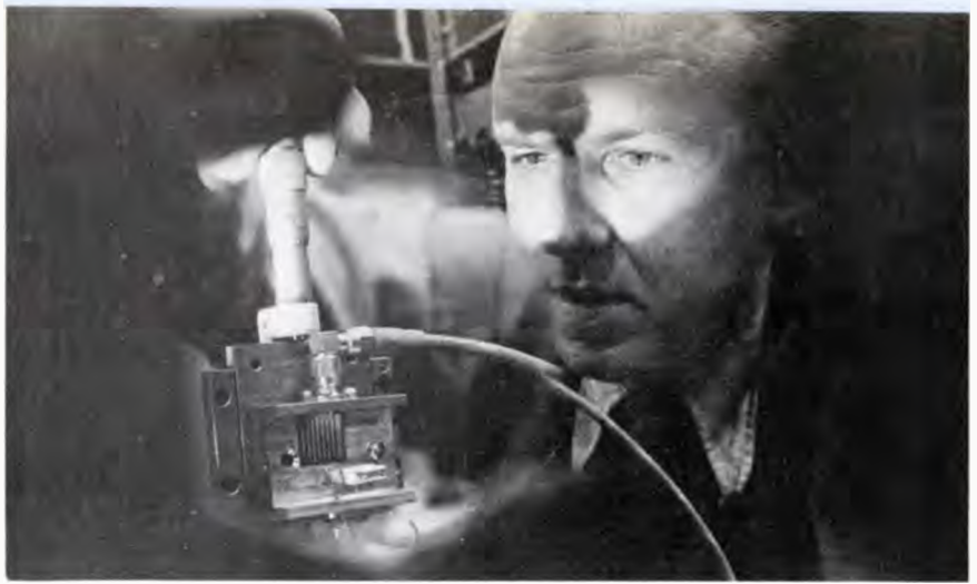
Switcher. Bell Labs' David Auston examines experimental setup that switches silicon in 10 picoseconds. The system could be made to work as fast as 1 ps, he says.
